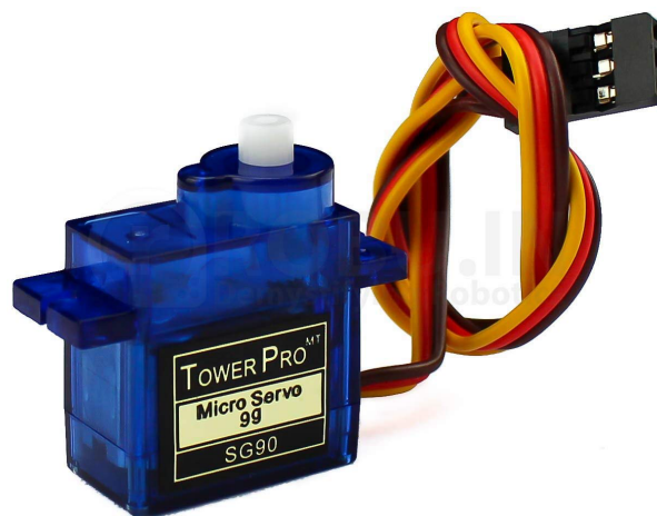
Slika 6: Servomotor Tower pro 9G
