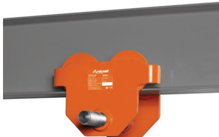
Slika 7. Kolica bez pogonskog lanca (Izvor: internetski portal [www.stuermer-machines.com](http://www.stuermer-machines.com))
