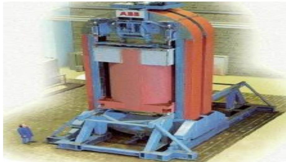
Slika 18. Kapsula HIP (**Hot isostatic pressing**)<sup>28</sup>
