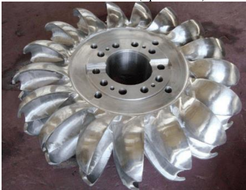
Slika 6. Pelton turbina (lopatice i rotor)
