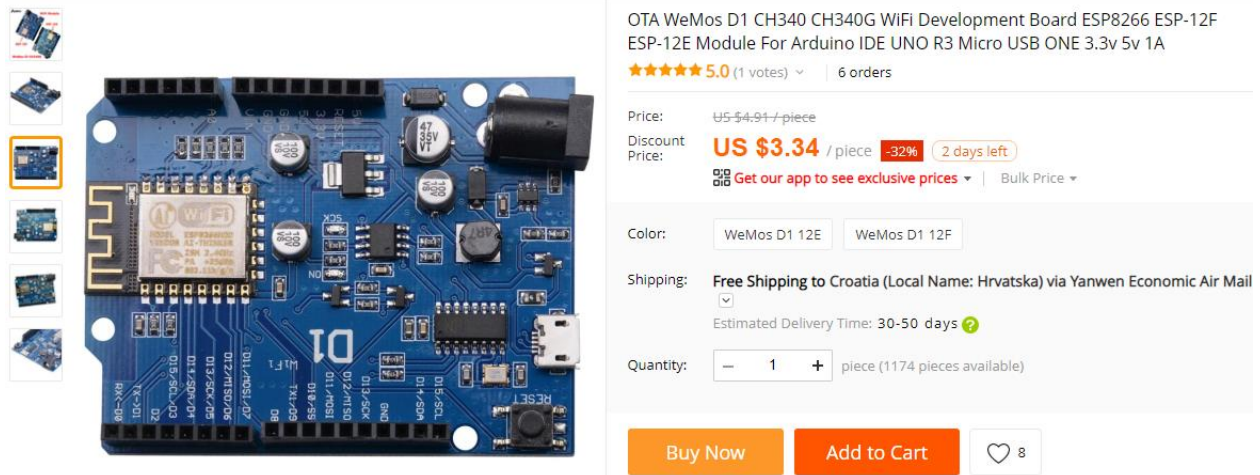
Slika 4: Wemos D1 Development Board ESP 8266
