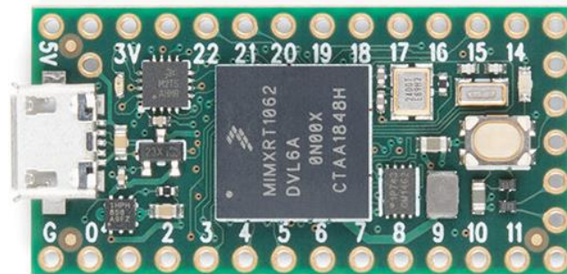
Slika 5. Primjer Teensy mikroupravljača. Preuzeto s https://www.electronics-lab.com/new-teensy-4-0-fastest-dev-board-powered-arm-cortex-m7/ .
