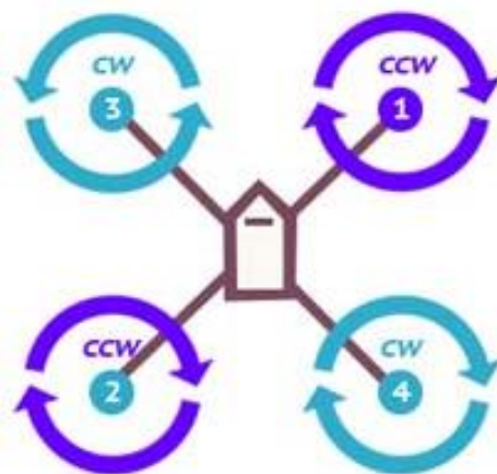
Slika 15. Primjer x-konfiguracije. https://circuitdigest.com/article/different-types-of-drone-frames-monocopter-to-octocopter
