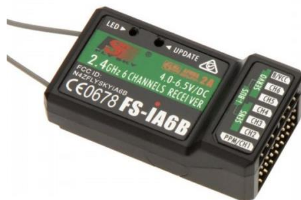
Slika 13. Primjer FS-iA6B. Preuzeto s https://alexnl.com/product/flysky-fs-i6-2-4g-6ch-afhds-rc-transmitter-with-fs-ia6b-receiver/
