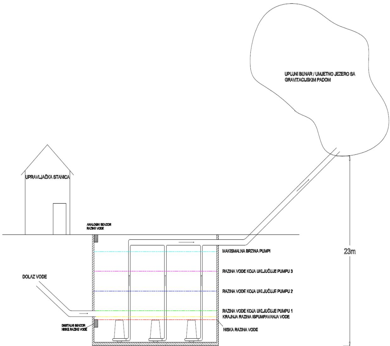
Slika 15. Blok shema pumpne stanice nacrtane u AutoCad softwareu
