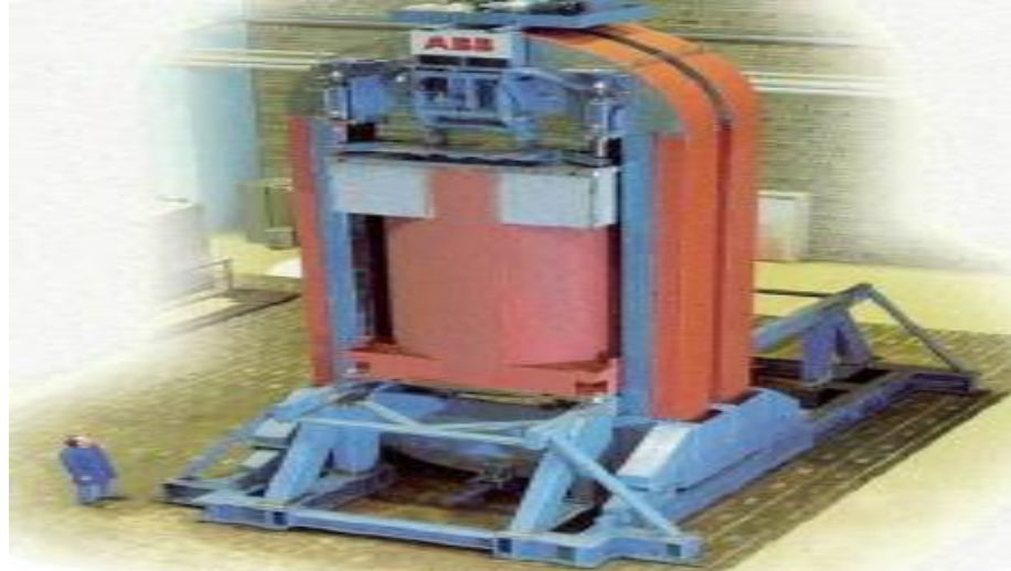
Slika 18. Kapsula HIP (Hot isostatic pressing) 28
