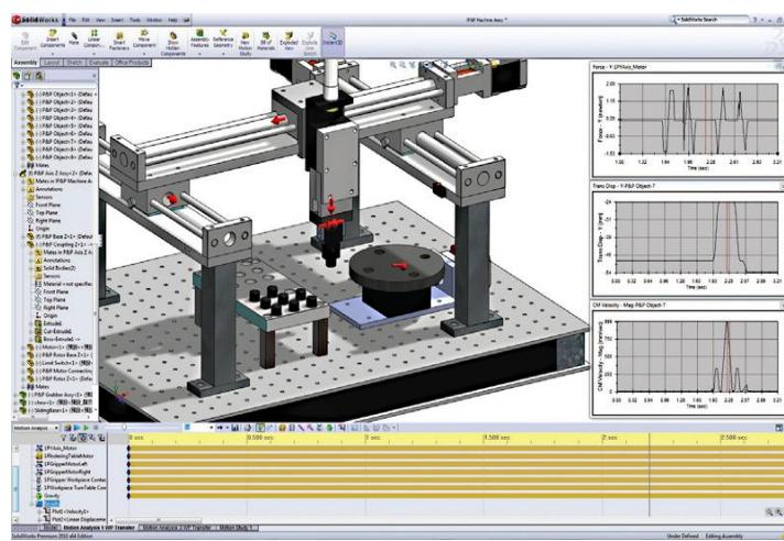
**Slika 12.** 3D virtualna izrada prototipova (3dcad virtual prototyping), Izvor: <https://www.3dcadworld.com/the-marriage-of-virtual-prototyping-and-mechatronics/>, 28.05.2022.
