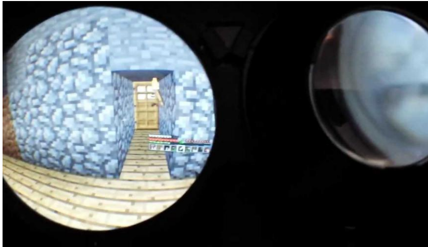
Slika 19. Efekt zaslonskih vrata (Screen Door Effect), Izvor: https://medium.com/nuadox/vr-screen-door-effect-21614df8f90e , 15.05.2022.
