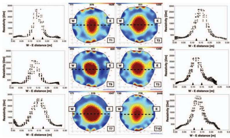
1. Electrical resistivity tomographs for the 10 trees. West to east profiles (from W to E) are plotted next to the tomographs. Dashed line the profile on the tomographs. Measured location of SW-HW boundaries are illustrated by triangles on the x-axis of the profiles.
