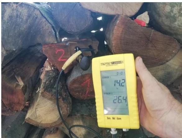
Slika 24: Mjerenje vlage bukove metrice. (Autor).
