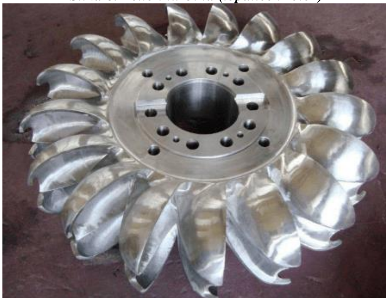
Slika 6. Pelton turbina (lopatice i rotor)
