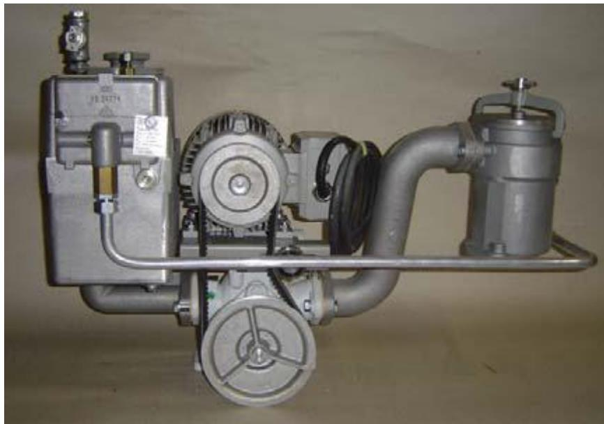
Slika 8: Sklop filtera, pumpe i separatora 9 lit, Izvor:<sup>18</sup>
